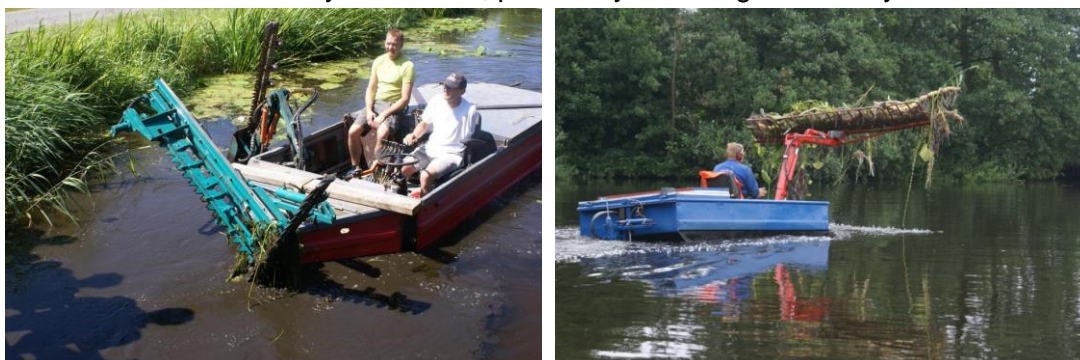
Figure 3.11: A weed cutting boat with adjustable mowing gear (left) and a harvesting boat (right) used for aquatic weed control in the Netherlands (Photos: R. Pot).
